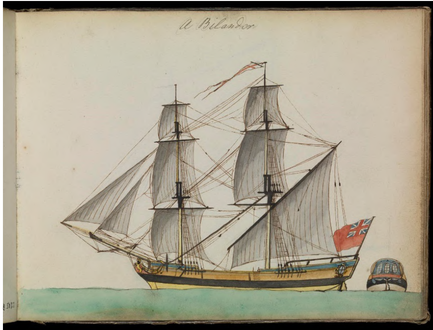
Figure 10. "British bilander showing sails and rigging and separate view of the stern" (c. 1780). Drawing by Edward Gwyn, © National Maritime Museum, Greenwich, London.
